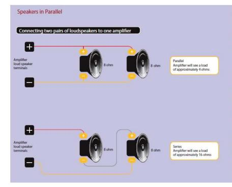
If you want to drive two pairs of loudspeakers from the output of one amplifier you can either connect them to a switchbox or wire them directly. If you use a switchbox then you can have the flexibility of listening to either or both pairs as required. If you always want both pairs to be active then it is possible to wire them directly as long as you are careful with the connections. There are two ways to wire the loudspeakers; either in series or in parallel.
